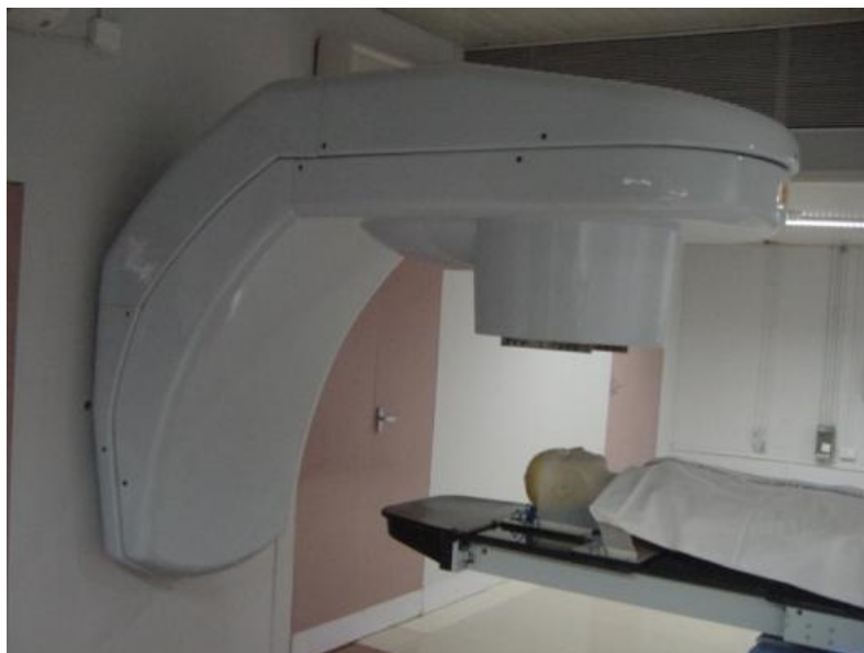
Figure 1: Bhabhatron-II tele-cobalt machine
