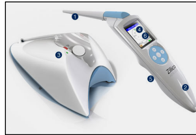
Fig.9: Prototype of tetrapolar probe for the detection of cervical cancer (by Zilico) in collaboration with Prof Browns's group.
